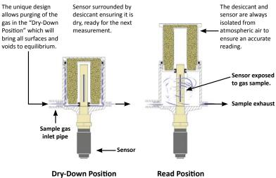
Keeping the sensor dry between tests ensures that the SDHmini is ready to carry out rapid spot checks. The unique design of the desiccant head achieves this by surrounding the sensor with desiccant, keeping the sensor dry. The head is then lifted for sampling, exposing the sensor to the sample gas.
